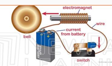
The magnetic field produced here when the circuit is closed is a combination of the magnetic force from the electrical current and the metal bar. Opening the circuit reduces the strength of the magnetic field and stops the clapper from striking the bell.
